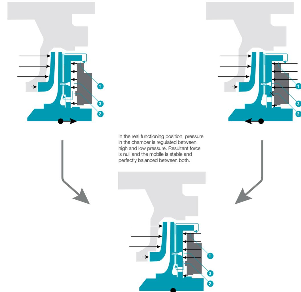
In the real functioning position, pressure in the chamber is regulated between high and low pressure. Resultant force is null and the mobile is stable and perfectly balanced between both.
